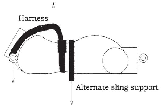
FIG. 3 Torso Support for Horizontal Position of the Torso
