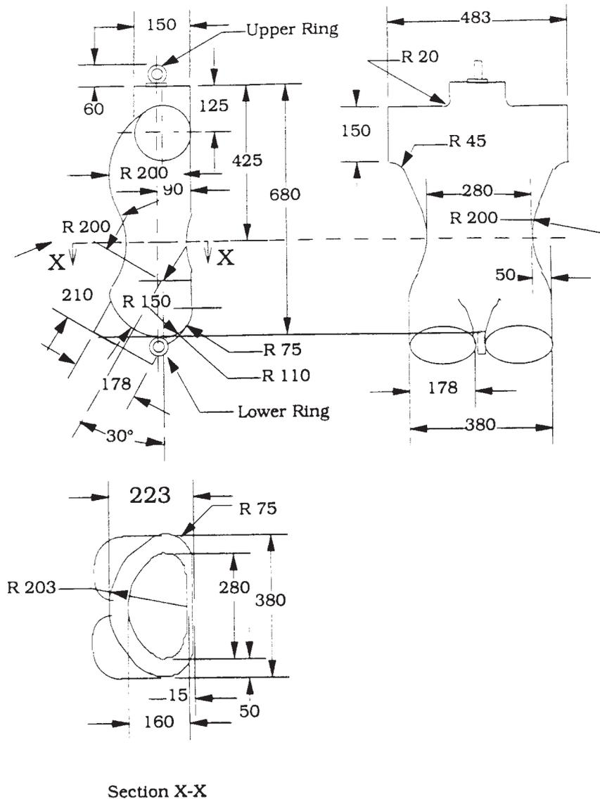
NOTE 1—All linear dimensions are in millimetres,  $\pm 5$  mm.
